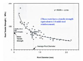
Fig. 4. Tensile strength of vetiver roots.
